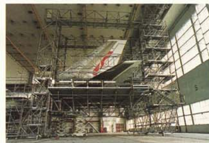
Universal tail dock for maintenance of any size passenger aircraft. This picture shows lifting of the working platforms by means of a chain drive. The equipment is in accordance with council directive 89/392 /EEC and therefore CE-certified. Inspection with final approval was carried out by DEKRA (German Quality Certification Authority) in Beijing in September 1997.
