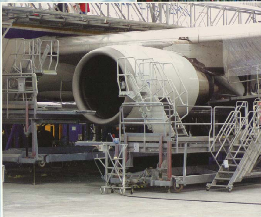
Nose- and tail dock module for A 320 aircraft in proven construction method for new maintenance hangar in Naples
