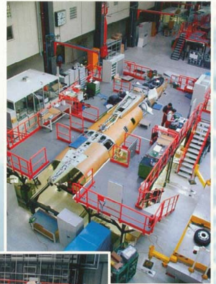
MERO aluminum building method - application at final assembly on Eurofighter in Manching (Germany)
